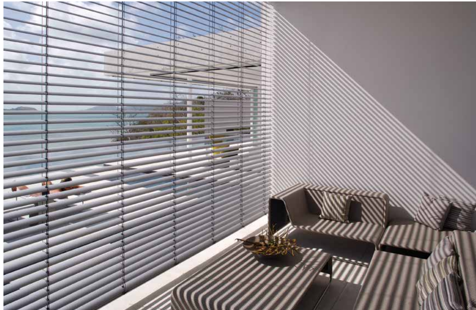
Above: Walls and shading devices are easily opened and adjusted to optimize air flow and moderate sunlight creating a comfortable environment that reduces the need for air-conditioning or artificial lighting.
